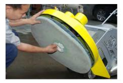
4. assembly back the clip cap ensure it is safety locked
