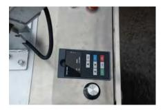
• Adjust the speed adjustable button to maximum speed(0-1800rpm). See above picture
