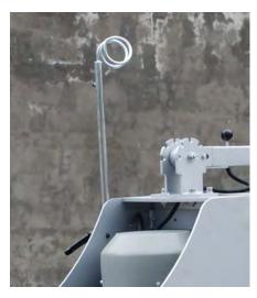
For safety and comfortable operation, please put the electrical wire on the wire hook.
