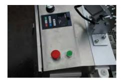
• Pull up the red emergency stop button, then push the green start button to Starting the machine. See above photo
